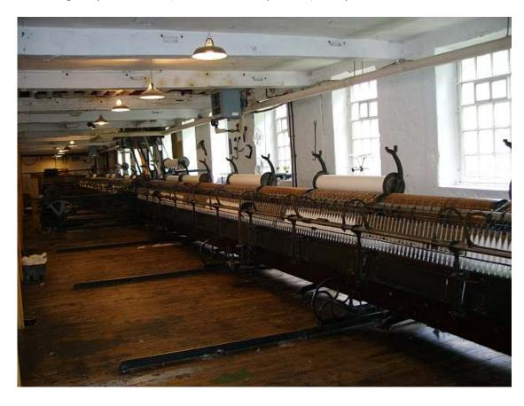
A working Mule spinning machine at Quarry Bank Mill 6
